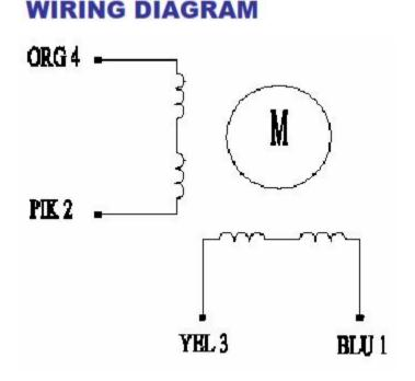
The bipolar stepper motor usually has four wires coming out of it. Unlike
